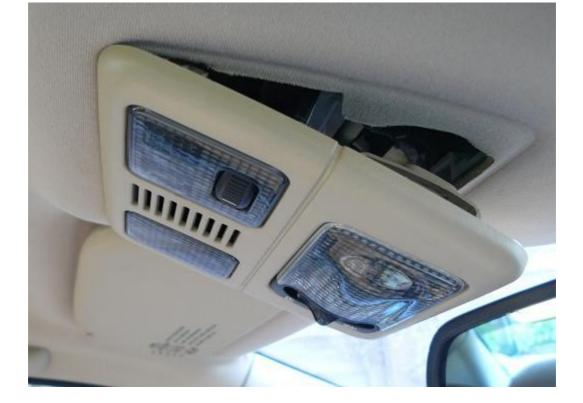
3. Next step is to remove the black fan unit from the console. First, detach its orange electrical connector. This was tucked up on the right hand side in the roof void.
