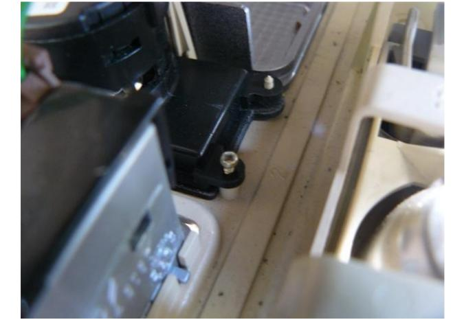
5. You should now have the back fan unit free to work on. I took mine in the house and found a small fine art brush to clean it. Here is the dirty before shot. You can see the air temperature sensor located out on two pins in the centre of the direction of airflow ... the fan is up behind it.
